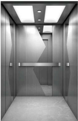
SH-K24 Side wall: Mirror stainless steel + Hairline stainless steel Rear wall: Mirror stainless steel + Hairline stainless steel Ceiling: Hairline stainless steel+LED lights Floor: PVC/Marble
